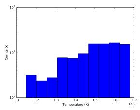
Figure 11 - Histogram maximum fuel temperature.
