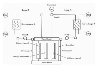
Figure 5 - Scheme of the TMI PWR benchmark.
