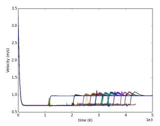
Figure 9 - Hot Leg flow velocity evolution.
